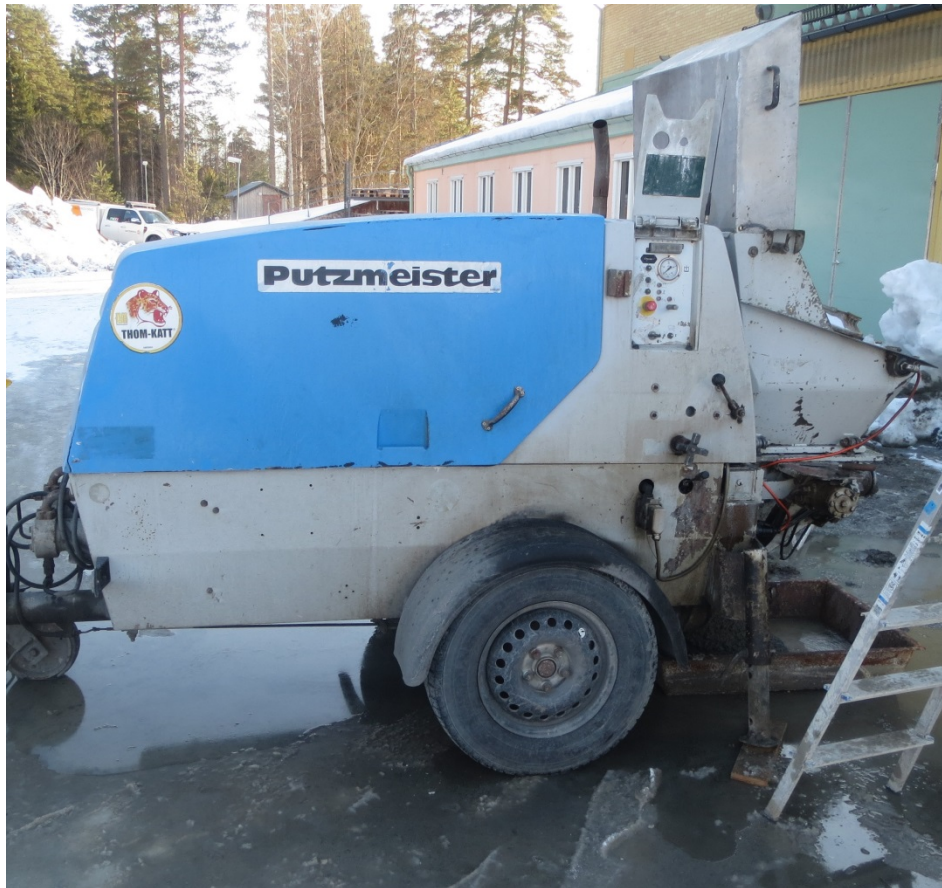
Figure 2.2 Concrete pumping machine, Putzmeister, THOM-KATT (TK 25).
