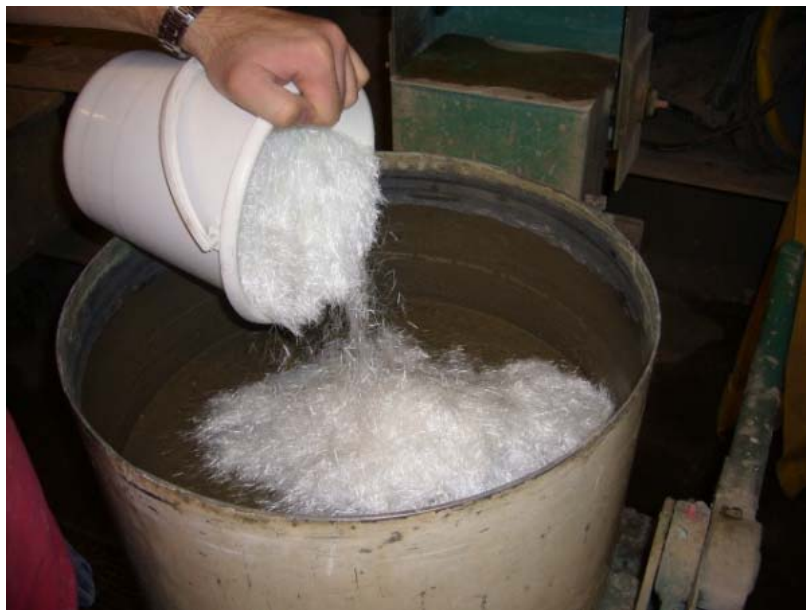
Figure 2.4. Micro fibres – here 6 mm long glass fibres.
