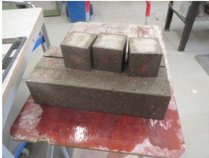
Figure 4.1. Test specimens from spray boxes, for compressive and flexural crack strengths tests.
