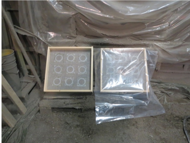
Figure 4.8. Special test boxes for bond strength tests.
